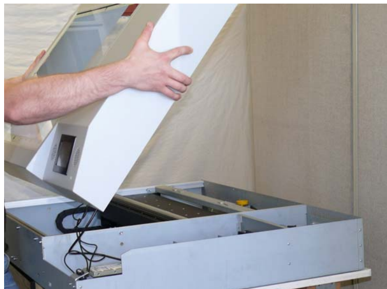
Picture 37: Separating device cover from device body
