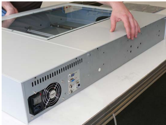
Picture 41: Device cover in end position
