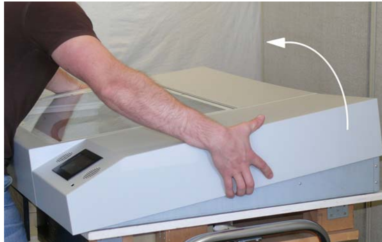
Picture 36: Lifting the device cover in arrow direction
