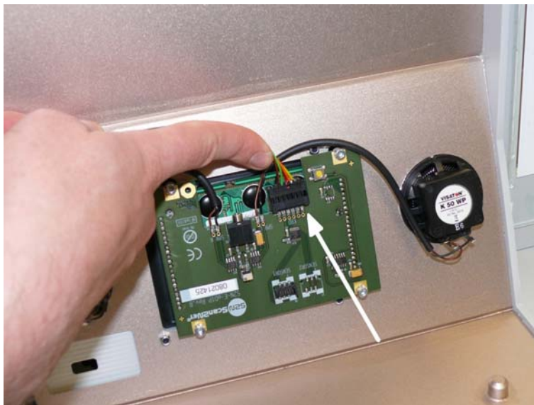
Picture 39: Disconnecting the signal cable
