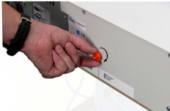
Picture 4: Inserting the transportation lock
