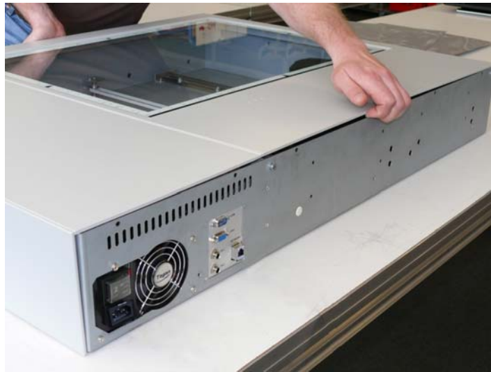
Picture 40: Lifting the device cover
