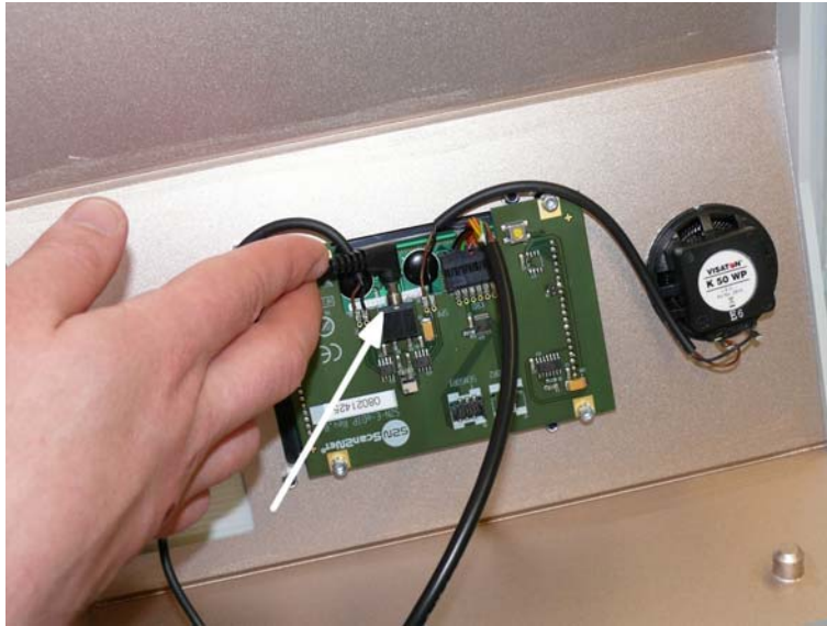
Picture 38: Disconnecting audio cable
