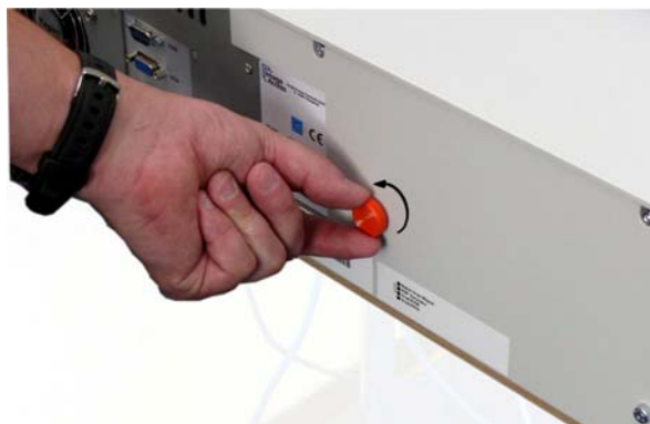
Picture 3: Removing the transportation lock
