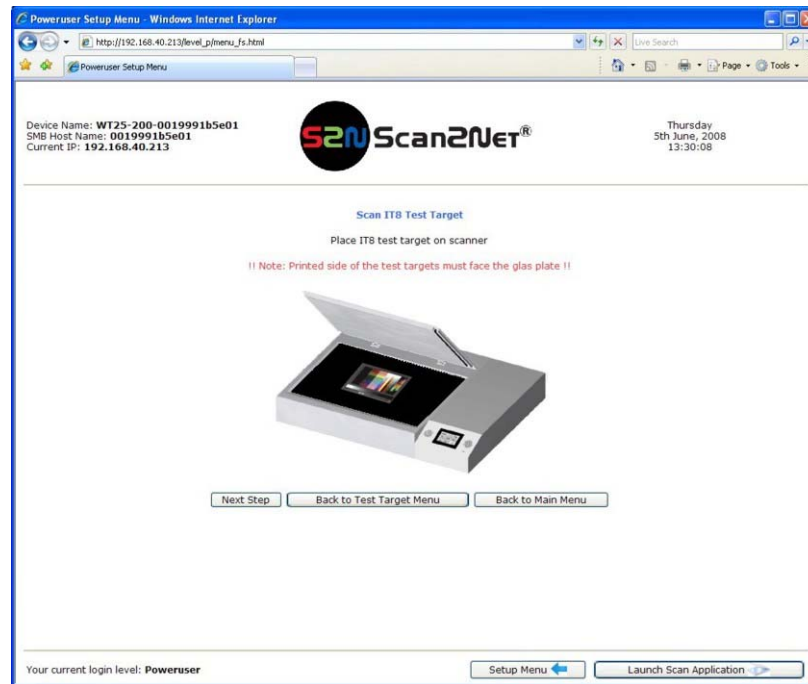
Picture 44: Position of IT8 test target on the glass plate
